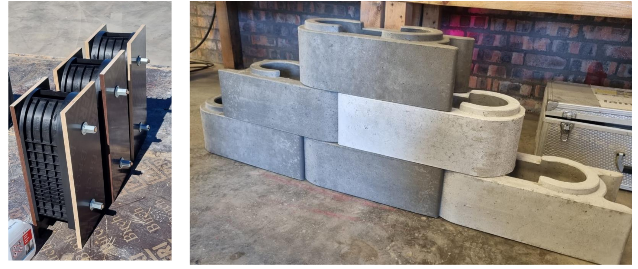
Above (left): TwistBlocks are made using special moulds produced by PERI, comprising of a recycled plastic form and two plywood closers. The newest version of moulds are now in production in South Africa and will produce much higher quality block than has previously been possible (above right).
